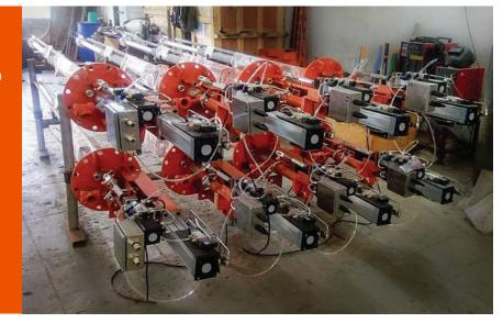
ZEECO Start-Up Burners (SUB) are designed for the reliable start-up of recirculating bed boilers. Utilizing high-energy direct spark ignition, ZEECO SUBs do not require a separate igniter train, increasing the overall system reliability. Featuring a dual cylinder
